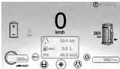
Simple Configuration in Extended Range Mode
